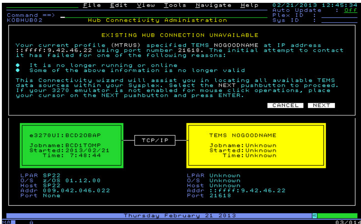
Figure 59. Hub Connectivity Administration workspace that shows a connectivity failure
